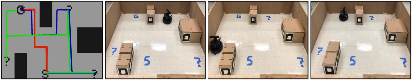
Figure 3: Demonstration of the path taken by the robot with three different initial beliefs for the map in Figure 1. The start state and the true goal state are denoted by S and G, respectively. The other potential goals are denoted by the question mark symbol. Green, blue, and red show the path taken by the robot with 0.1, 0.25, and 0.9 as the initial belief for the true goal state and equal probability for other potential goal states.
